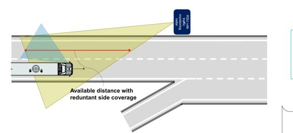
Distance with redundant side coverage from on-board and off-board sensors. Sensor ranges and angles are not to scale.
